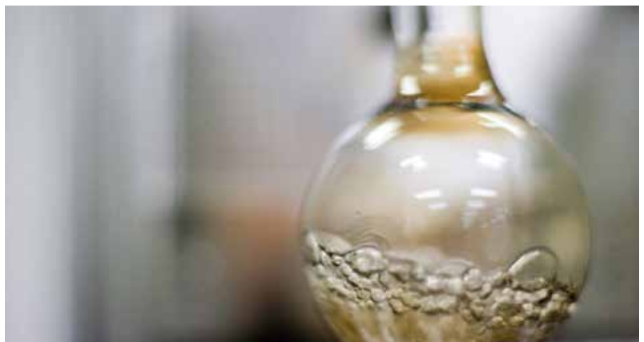
FIGURE 2: The formation of air bubbles in an oil formulation.
