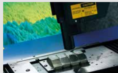
FIGURE 11: The optical profilometer uses a laser as a non-destructive way to measure wear. It is enabling Shell scientists to evaluate product wear performance more precisely than conventional methods.
