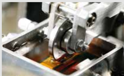
FIGURE 10: The unique slide/roll rig test, which was designed by Shell, is a good simulation of diesel engine wear tests. It is used to screen a wider range of candidate oil chemistries in a shorter time than full engine tests would enable. The best technologies are then tested further in selected engine tests.
